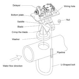
Figure 2 Installation Drawing
