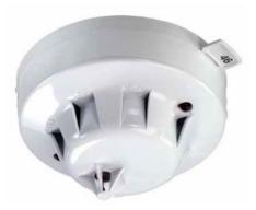
The Discovery CO/Heat Multisensor Detector contains a CO detection cell and a thermistor temperature sensor whose outputs are combined to give the final analogue value. The way in which the signals from the two sensors are combined depends on the response mode selected. The CO/ Heat Multisensor detects the presence of carbon monoxide or heat or a combination of both.
