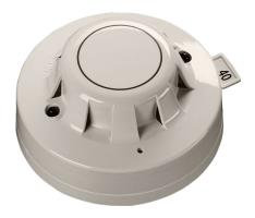
The Discovery Ionisation Smoke Detector uses the same outer case as the optical smoke detector and is distinguished by the red indicator LEDs. Inside the case is a printed circuit board which has the ionisation chamber mounted on one side and the signal processing and communications electronics on the other.
