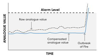
Figure 1 – Drift Compensation Graph
