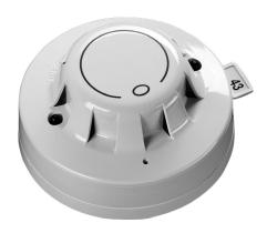
Discovery CO fire detectors contain a long-life electro-chemical carbon monoxide sensor which is tolerant of low levels of common vapours and household products. The sensing technology is fast, accurate and needs only very low power. The detection capabilities are enhanced by a rate sensitive response. Fast rises in the carbon monoxide level are often associated with hot fires and the detector will respond earlier under these conditions.
